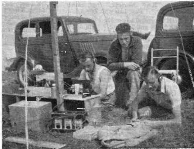
Yes, this was in the old days! G2AK, G8MC and G3FD (l. to r.) operating portable at Brixham in 1937. The Tx, a 42-6L6 in CO/Tritet-PA, is still in use and covers all bands 1.7 to 28 mc; the modulator is 6N7-P/P 6N7. The whole outfit is powered from a 300-volt 150 mA converter run off the 12v. car battery. The Rx at the time was a straight 1-V-1.
